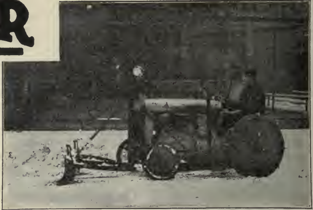
Special Snow Plow for Fordson Tractor
